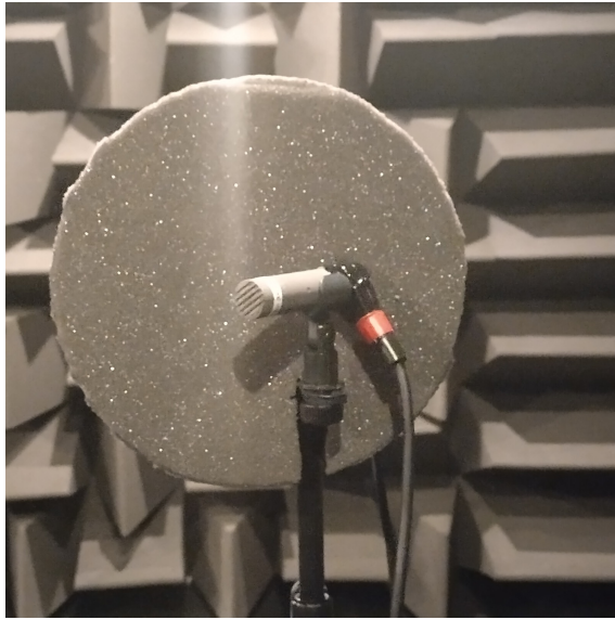
(a) SCHOEPS MK2 16 spherical response microphone, -45^\circ ; a baffle disc of acoustic foam 17
